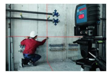
Figure 6 An alignment laser
